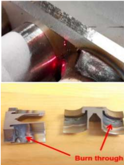
Laser searching disturbed by spatter and tubes affected by too much heat
